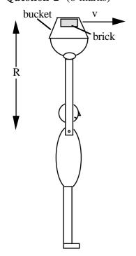
A physics lecturer swings a bucket in a vertical circle, radius R, about his shoulder, as shown. The bucket contains a brick. Determine the minimum speed v that the bucket must have at the top of the circle so that the brick stays in contact with the bucket?
