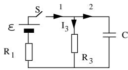
In the circuit shown at left, the capacitor C is initially uncharged and the switch S is open.
