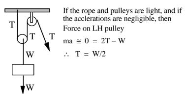
If mass rises by D, word done = WD. But rope shortens on both sides of rising pulley, if mass rises by D, rope must be pulled 2D, so work done =  $T \times 2D = WD$
